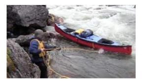
**Definition:** a line looped around the front end of the canoe to which another is attached unde the canoe and used for towing the craft.
