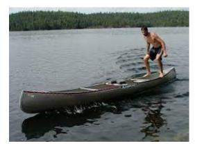
**Definition:** the section along the top of the canoe from stern to bow where the sides meet; a strip along the top of the canoe's sides.
